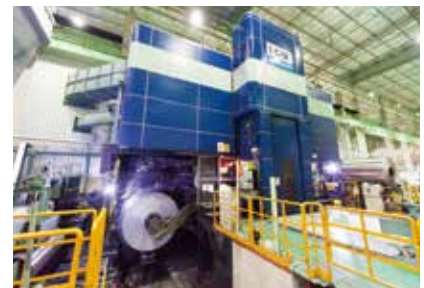
Six-high cold rolling mill
