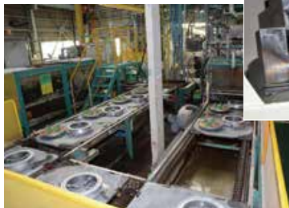
Plaster mold production line
