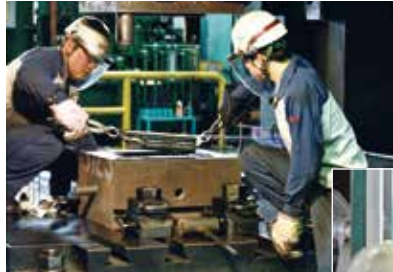
Die forging process
