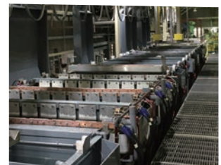
Anodized surface treatment line
