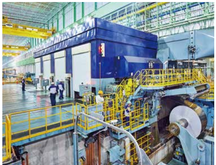
Four-stand hot finishing rolling mill
