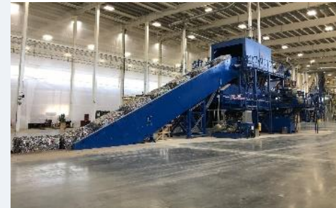
(1) Crushing compressed UBCs
