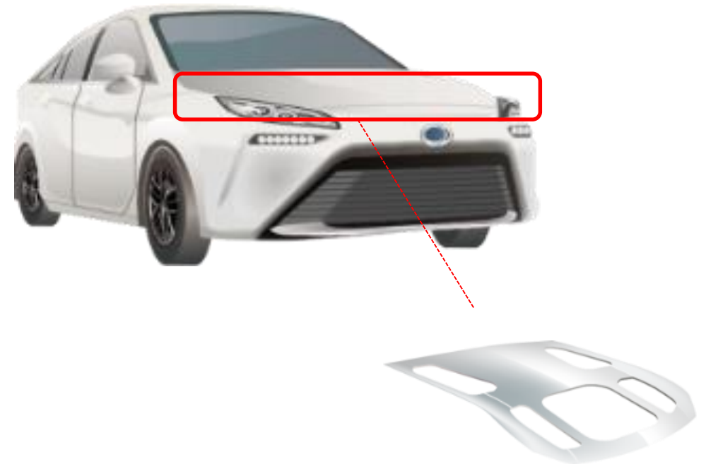
Recycled aluminum material is used for hood inners
