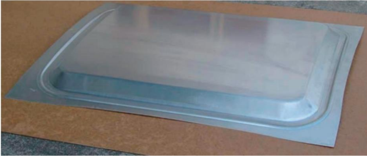
Figure 1: Experimental press mold for 6000 series development alloy sheet
