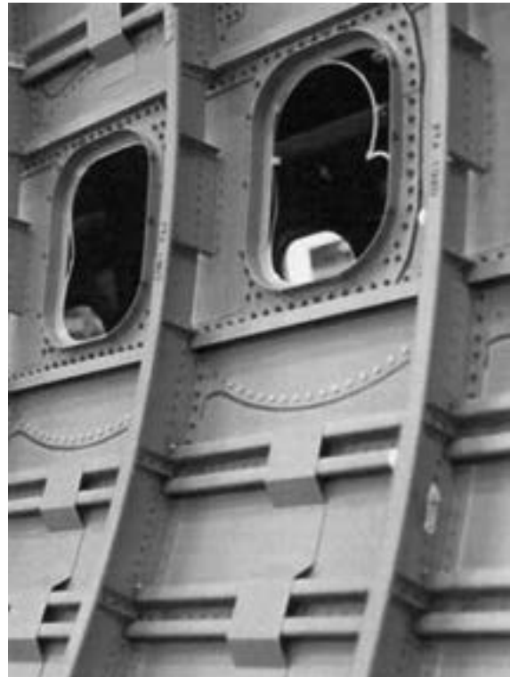
Fig. 6 B767 and its fuselage constructed with frames, skins and taper-rolled stringers 24), 25) .
