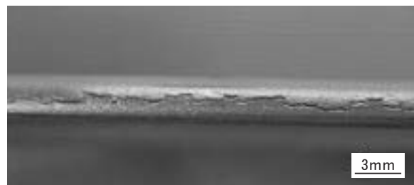
Fig. 1 Appearance of hem cracking.
