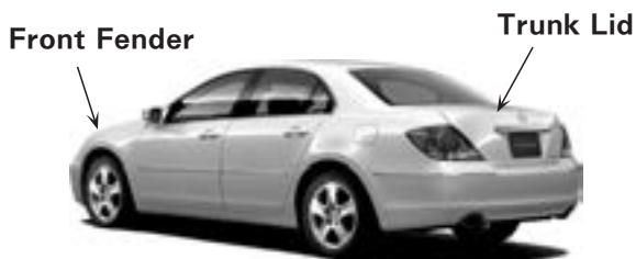
Fig. 7 Aluminum body panels applied superplastic forming on Honda Legend (Acura RL) 19) .
