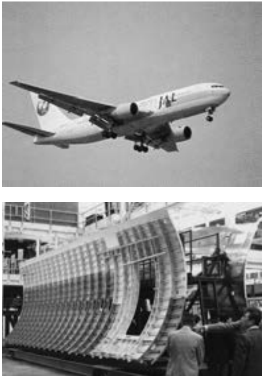
Fig. 6 B767 and its fuselage constructed with frames, skins and taper-rolled stringers 24), 25) .
