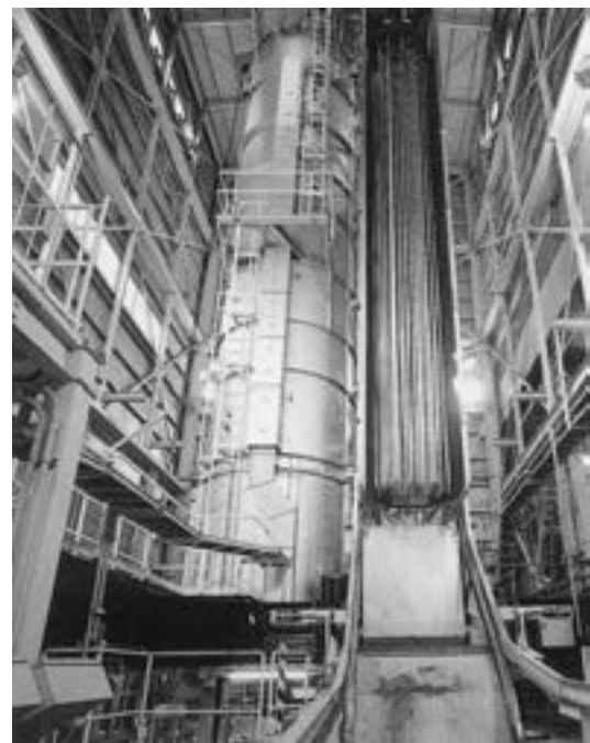
Fig. 22 Vertical furnace with quenching medium of polyalkylene glycol 62), 63) .
