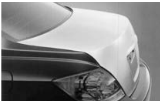
Fig. 26 Fender and trunk-lid of Honda Legend produced by high speed blow forming 84) .
