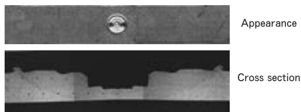
Fig. 8 Joint of Friction Stir Spot Welding (6000 series alloy sheets for automobile body).
