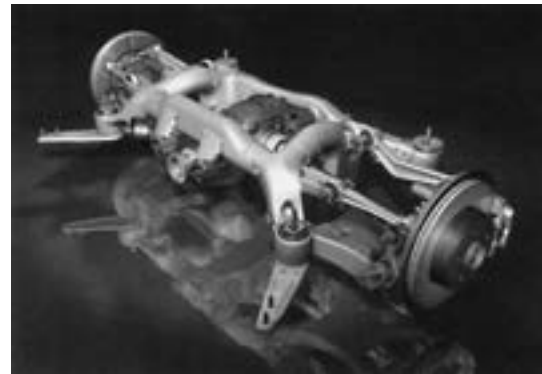
Fig. 9 Rear suspension on BMW 5 series(E60) 37) .
