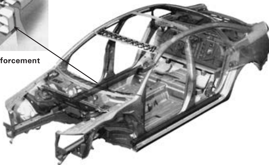
Fig. 6 Side sill reinforcement of Audi A6 (C6) 16) .
