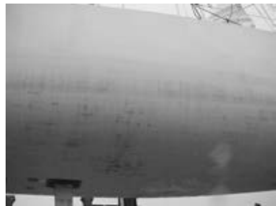
Fig. 4 The paint condition of the external surface of "SUNTORY-Mermaid".
