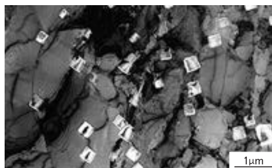
Fig. 13 TEM image of initial pits formed at subgrain boundaries.
