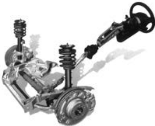
Fig. 7 Front suspension on BMW 1 series 28) .
