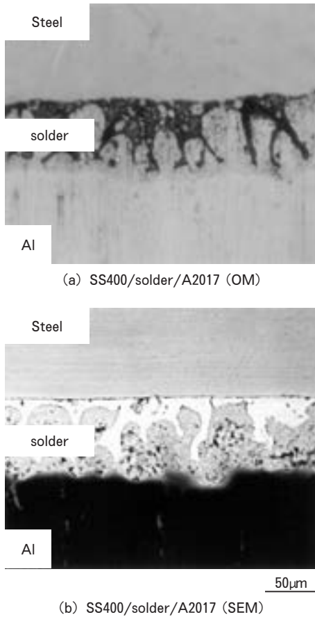
Fig. 9 Optical micrograph and scanning electron micrograph of the cross section of SS400/2017 joint bonded.
