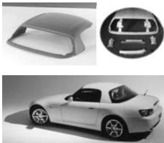
Fig. 11 Honda S2000 and its removable roof 44) .
