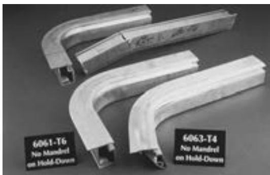
Fig. 3 Examples of retrogression bending of large, hard-tempered and complex truck door frames 6) .
