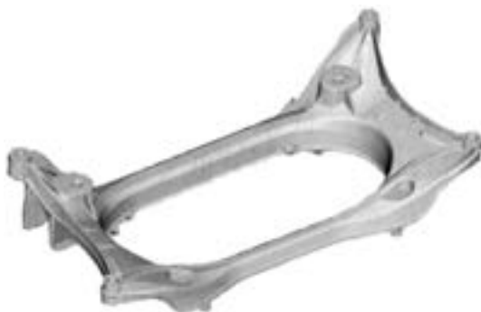
Fig. 8 Front suspension member on Toyota Crown 35) .
