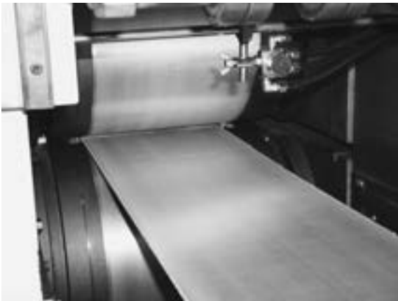
Fig. 2 An example of twin roll casting strip 2) .
