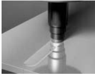
Fig. 6b Friction stir welding (FSW).
