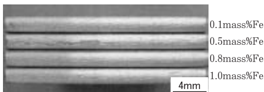
Fig. 9 Appearance of the bent specimens. Bending direction is parallel to the rolling direction and the radius is 0mm.
