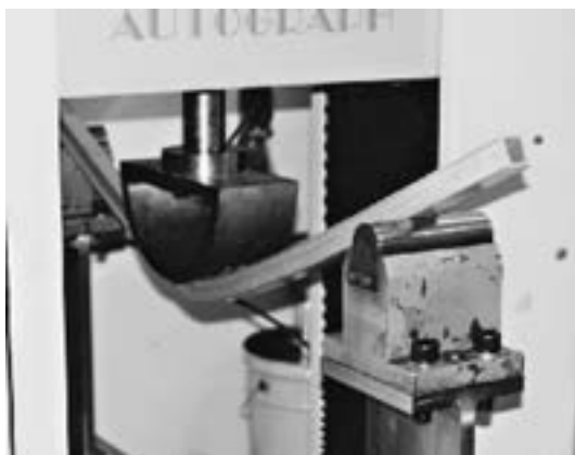
Fig. 9 3-points bending test.
