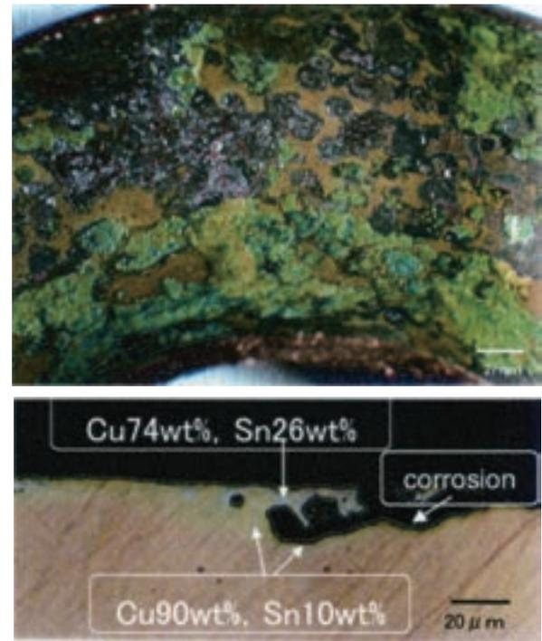
Fig. 2 Appearance of inner surface, cross section and EPMA analysis of the tin coated U-bend tube at heated portion by brazing. Sample tube was tested for 4 months in Test 1.
