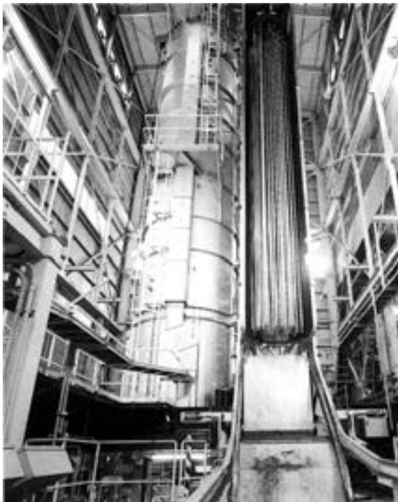
Fig. 36 Vertical quenching furnace.
