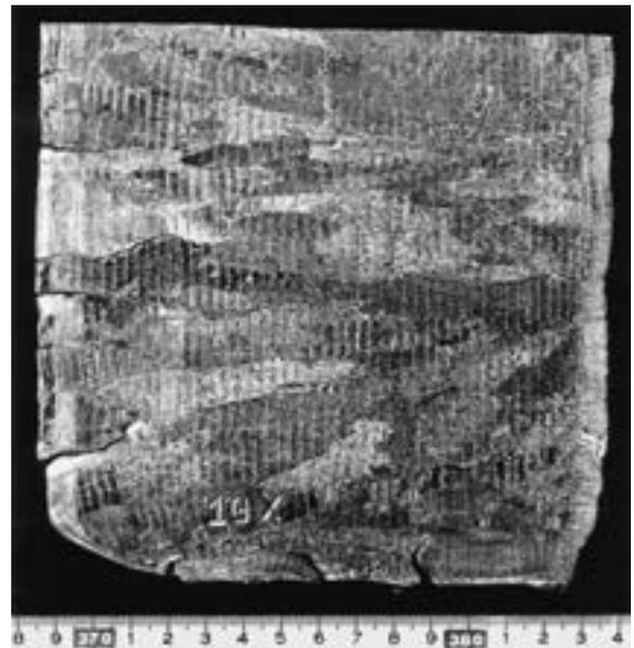
Fig. 40 Intergranular fracture of hot rolled sheet in 99.99% Aluminum<sup>58)</sup>.
