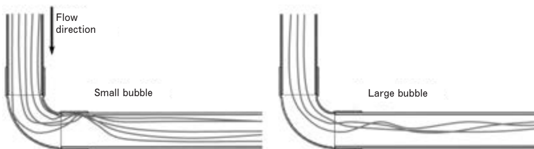
Fig. 6 Typical illustration of bubbles flow nearby elbow in the transparent tube at flow rate of 1.5m/s.
