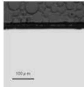
(a) Gap between specimen and epoxy resin
