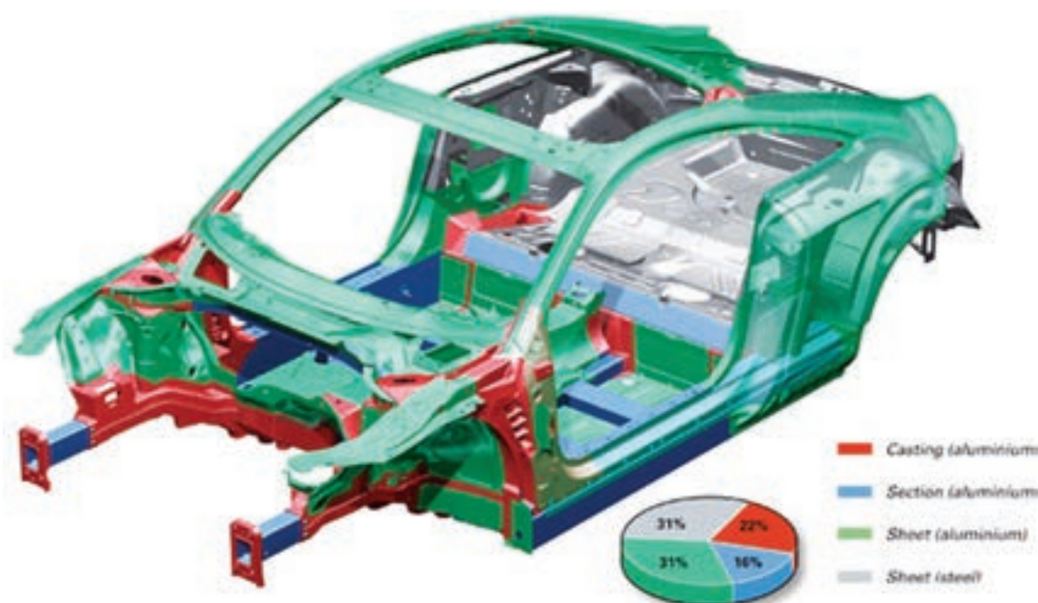
Fig. 9 Hybrid space frame of Audi TT coupe 11)
