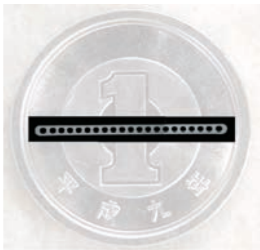
Fig. 1 Example of the cross section of multi flow tube for condenser of car air conditioner
