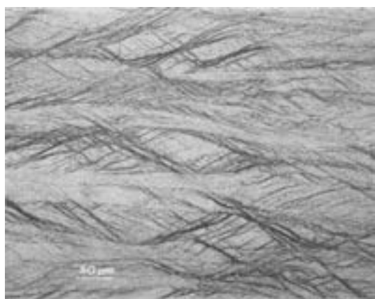
Fig. 33 Shear bands in cold rolled Al-4.5%Mg alloy 81) .
