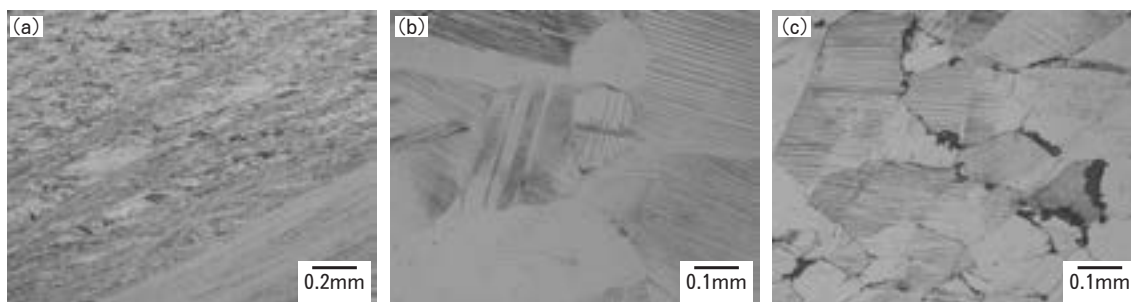
Fig. 2 Microstructures of forged Cu-3 mass%Ti alloys at (a) 773K, (b) 823K and (c) 873K.
