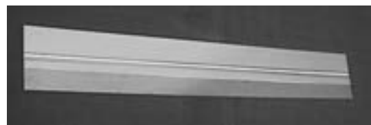
Fig. 11 Seam welding joints of aluminum/steel sheets for 1 m long.
