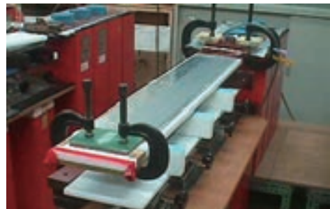
(b) Sheets for welding put on insulated above coil.
