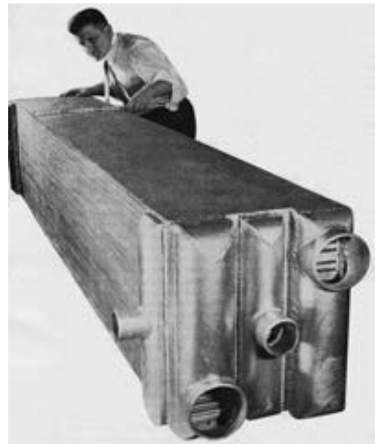
Fig. 3 Large heat exchanger brazed by dip brazing. 14)
