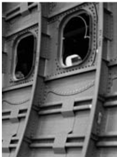
Fig. 44 Fuselage of B767 made of taper-rolled stringer 4,5,44) .
