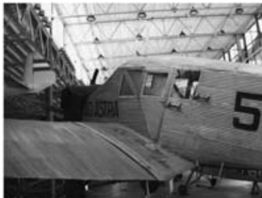
Fig. 2 Yunkers F.13 fabricated with corrugated panels of Duralumin sheets ( http://www.idflieg.com/junkers-f13.htm , ©2006 Andi Szekeres)
