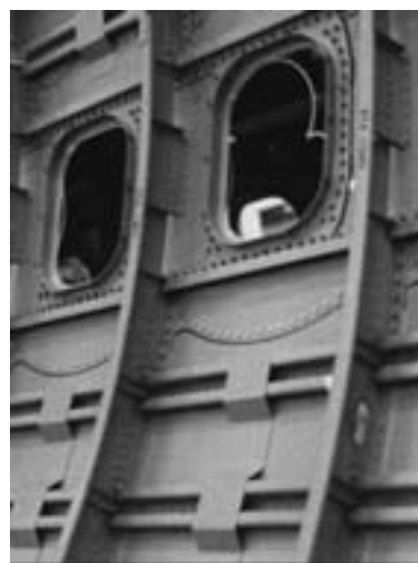
Fig. 12 B767's fuselage constructed with frames, skins and taper-rolled stringers
