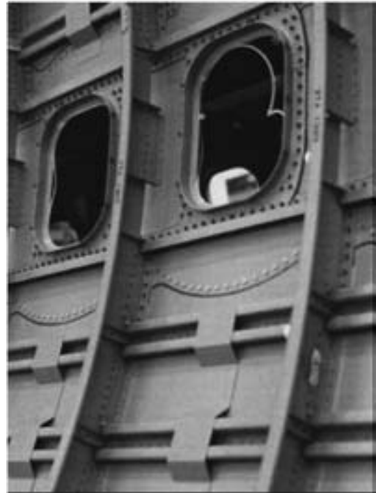
Fig. 42 B767's fuselage constructed with frames, skins and taper-rolled stringers 99, 104)
