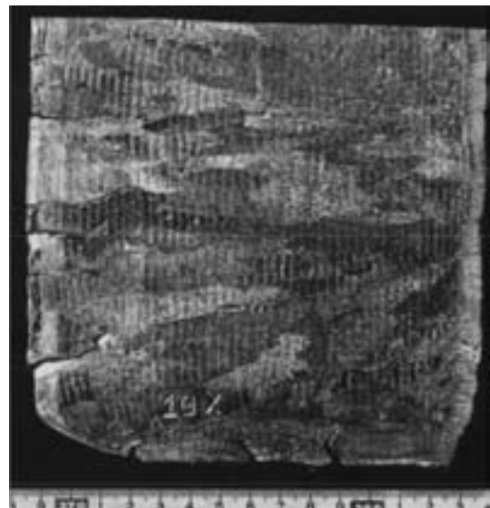
Fig. 22 Intergranular fracture of hot rolled sheet in 99.99% aluminum 26) .
