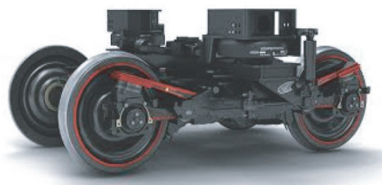
Fig. 13 Cart made of carbon fiber composite material (Kawasaki Heavy Industries: efSET) 17) .
