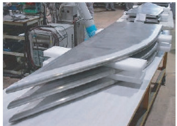
Fig. 7 Pantograph cover made by honeycomb sandwich panel on Shinkansen.
