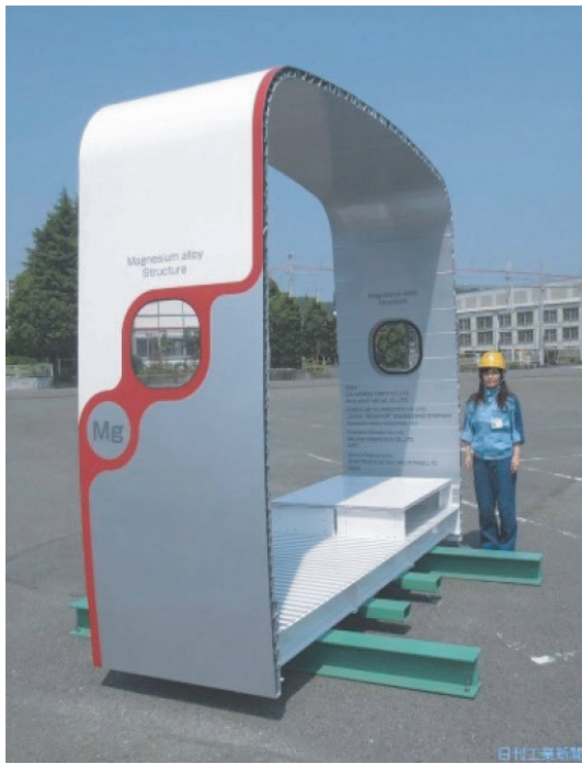
Fig. 14 The simulated structure of car vehicles on flame-retardant magnesium alloy 18) .
