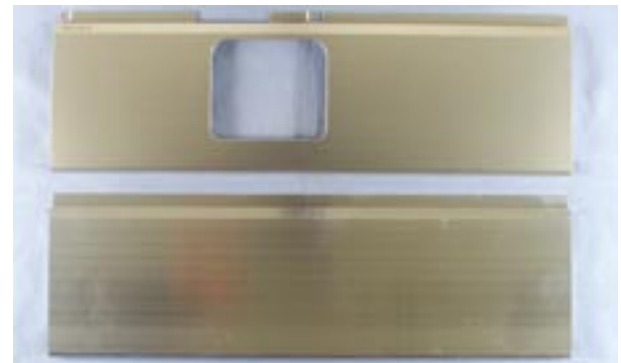
図7 アルミニウム押出型材 Fig.7 Extruded bar(Upper: After hairline treatment, Lower: Extruded aluminum shape).
