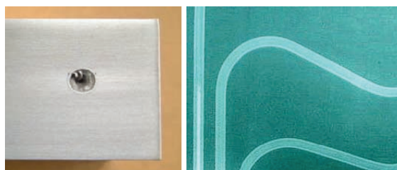
図14 ヒータ部断面と透過X線写真 Fig.14 Cross section and transmission X-ray photograph of heater.
