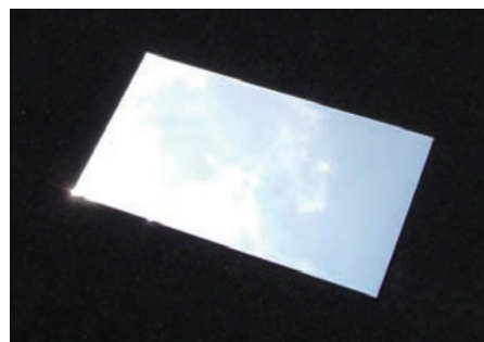
図2 屋外仕様の光ダクト用反射板の外観 Fig.2 Appearance of outdoor-type reflector for mirror duct.
