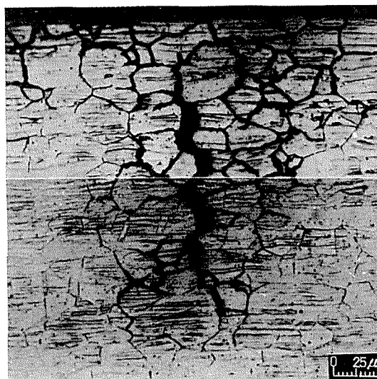
Fig. 18 Cross section of 30% cupronickel by exposure to degassed steam at 350°C for 500 hours under applied tensile stress of 18.5 kg/mm 2 , showing the intergranular cracking by tensile stress.
