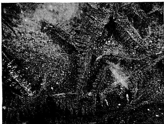
Fig. 10 Typical 3-dimensional dendrites ( \times 16 ). Electrolysis condition : G-17 in Table 1.
