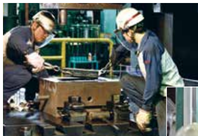
Die forging process
