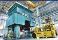
15,000t large-scale forging press
