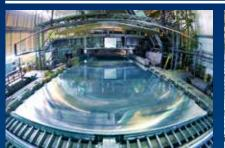
400m long rolling mill dedicated to producing only LNG tanker aluminum thick plates in Japan
