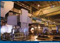
Rolling mill capable of producing 2m-wide coils with outer diameter over 2m
