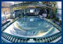
400m long rolling mill dedicated to producing only LNG tanker aluminum thick plates in Japan
