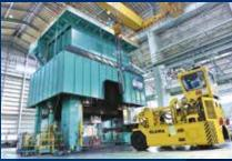
15,000t large-scale forging press
