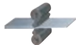
Hot mill rough rolling
