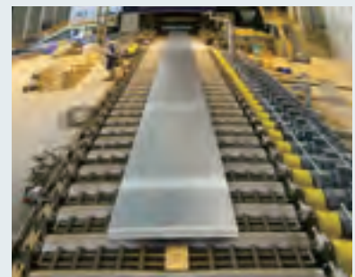
Hot mill rough rolling
