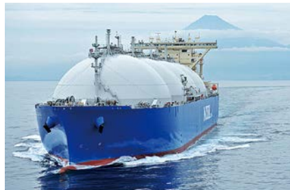
1970 | Transport ships Japan's first aluminum thick plates for LNG carrier storage tanks manufactured
