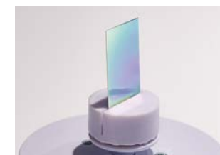
"Rainbow anodized aluminum" changes color depending on the angle of light.
