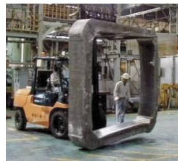
図5 大型自由鍛造品(液晶装置用) Fig.5 Large-scale free forging (for LCD).
