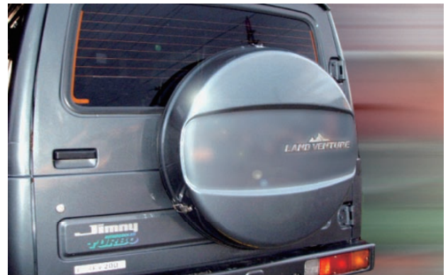
図10 車載タイヤハウス Fig.10 Spare tire housing for SUV.
