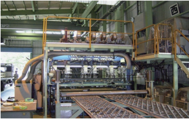
図7 プレリブ連続溶接機 Fig.7 Continuous welding machine.
