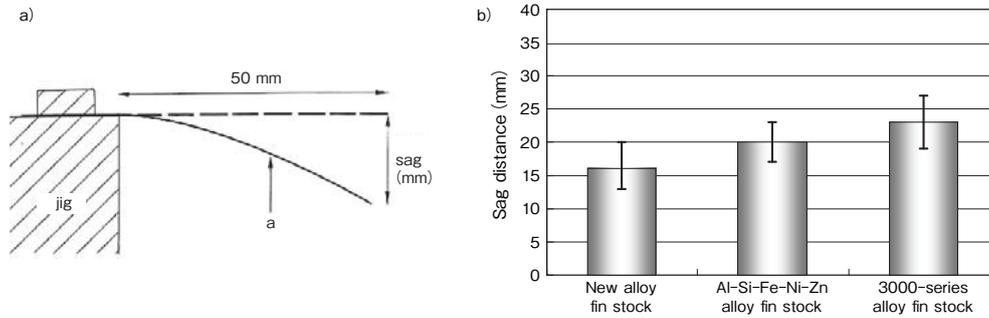
Fig.8 a) Sag test apparatus (arrow a indicates a specimen)
