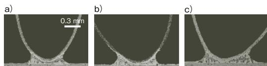
**Fig.7** Cross section of a fin-tube joint.
