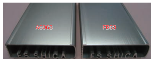
図2 「A6063」と「FB63」との外観比較 Fig.2 Appearance comparison between “A6063” and “FB63”.
