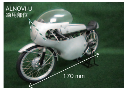
図6 ALNOVI-U適用部品 (エムエムピー社ミニチュアバイクのカウリング) Fig.6 Midget component made of ALNOVI-U by blow forming (Cowling of midget bike by MMP. Co.)
