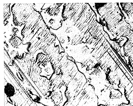
Photo. 7. Microstructure of Ti-36% Al alloy. Arc cast structure, \gamma and \delta phases.
