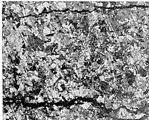
Photo. 5 Typical stress-corrosion crack in Albrac pipe tested in cooling water of transformer oil for two years.
