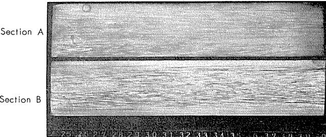
b) Parallel sections to extruded direction.
