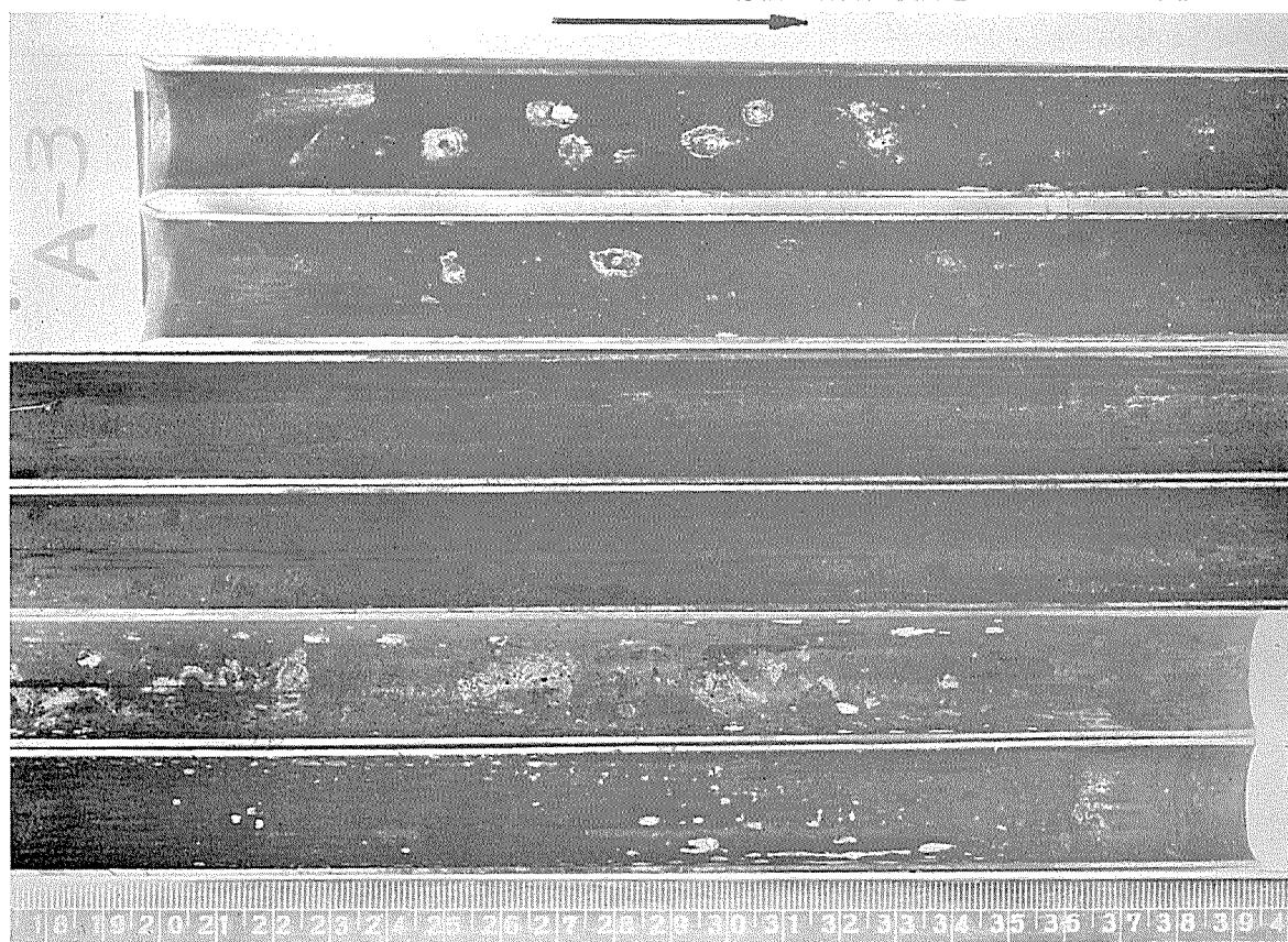
Photo. 2 Scales formed on aluminium brass tube.
