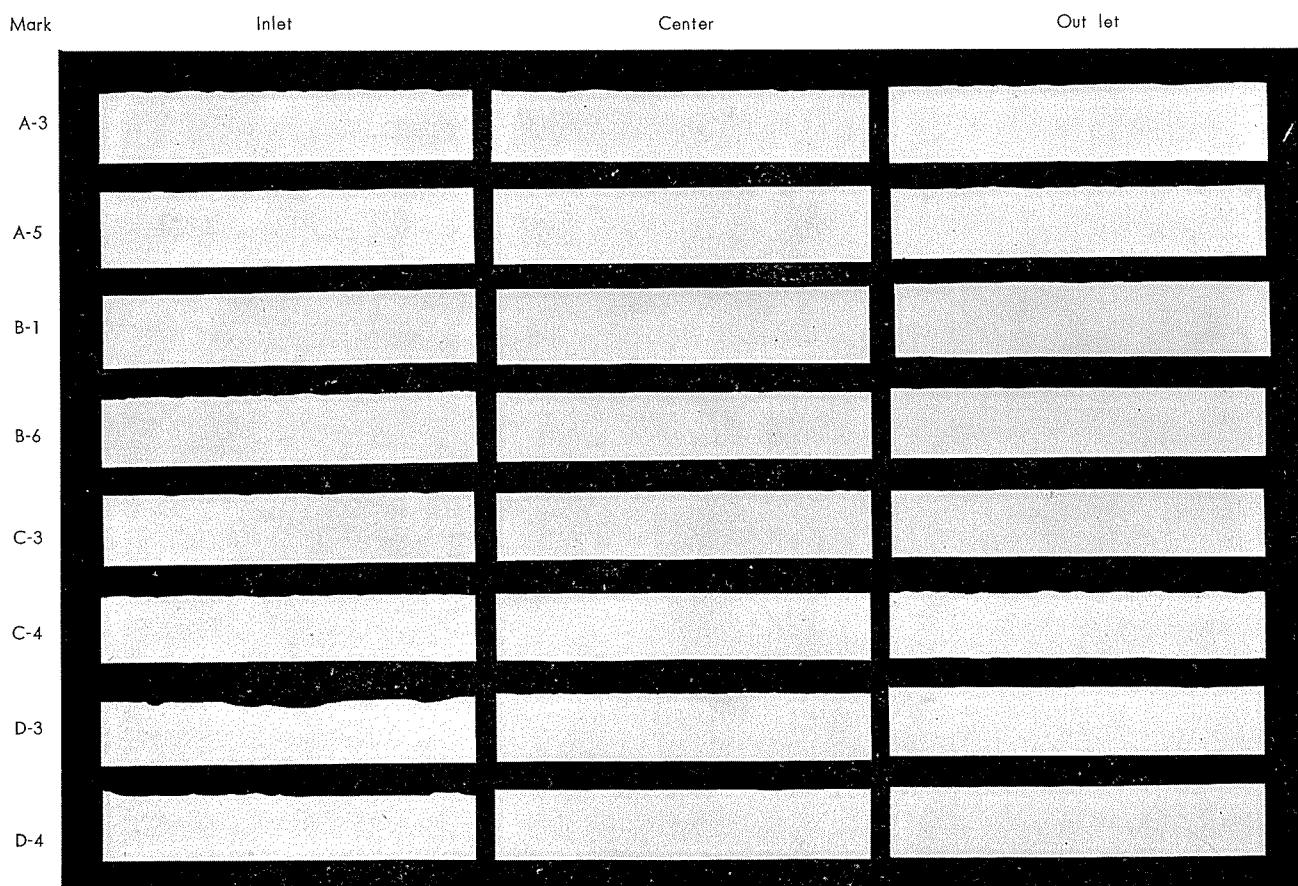
Photo. 4 Longitudinal cross sections of test tube. (duration of test: March~September 1958, 3822h) ×8
