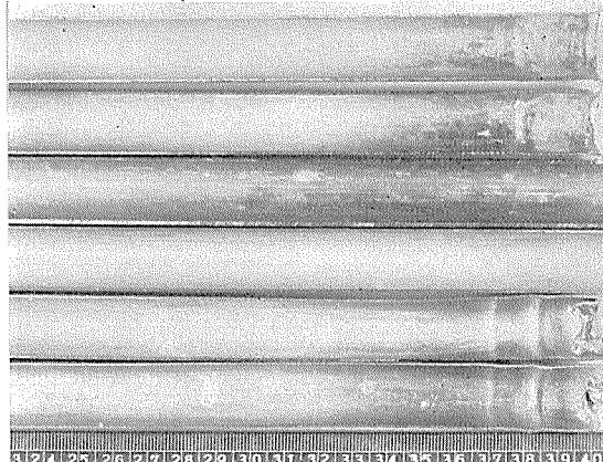
Photo. 14 Inner surface of Albrac tube.(Work hardened)
