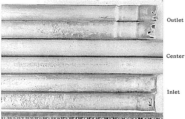
**Photo. 6** Inner surfaces of arsenical admiralty brass tube.
