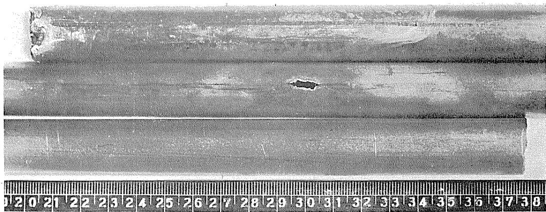
(a) Crack of 90-10 cupronickel tubes.
