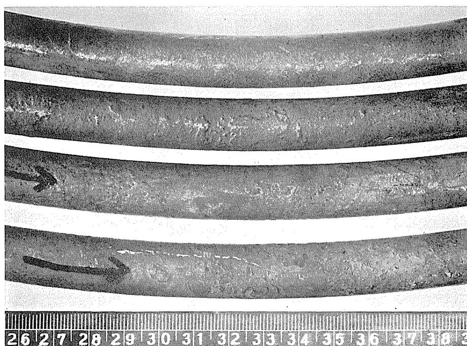
(a) Exfoliation corrosion on the outer surface.
