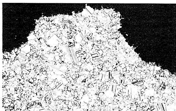
(a) Corrosion by heavily polluted sea water at O Power Station.
