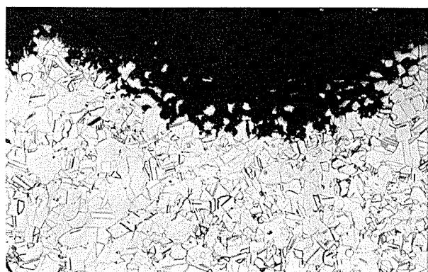
(b) Corrosion by slightly polluted sea water at S-N Power Station.
