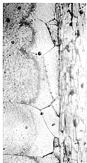
Photo. 1 Micro structure of clad part of Alclad 7075 alloys after solution heat treatment. (×280)
