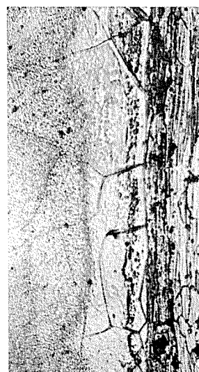
Photo. 5 Micro structure of clad part 1.07% Mg added of Alclad 7075 alloys after solution heat treatment. (×280)
