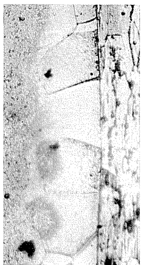
Photo. 1 Micro structure of clad part of Alclad 7075 alloys after solution heat treatment. (×280)
