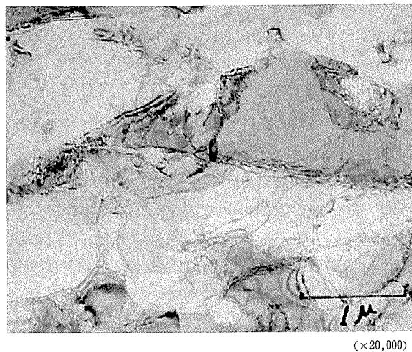
**Photo. 5** Transmission electron microstructure of commercial aluminum annealed at 150°C after 90% cold rolling.
