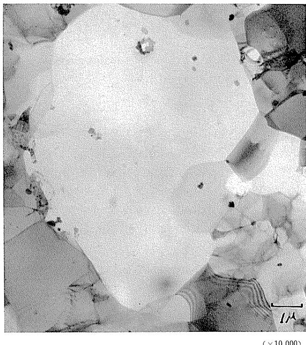
**Photo. 11** Transmission electron microstructure of commercial aluminum annealed at 250°C after 90% cold rolling.
