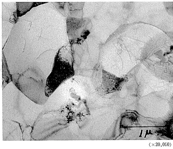
**Photo. 6** Transmission electron microstructure of commercial aluminum annealed at 200°C after 90% cold rolling.
