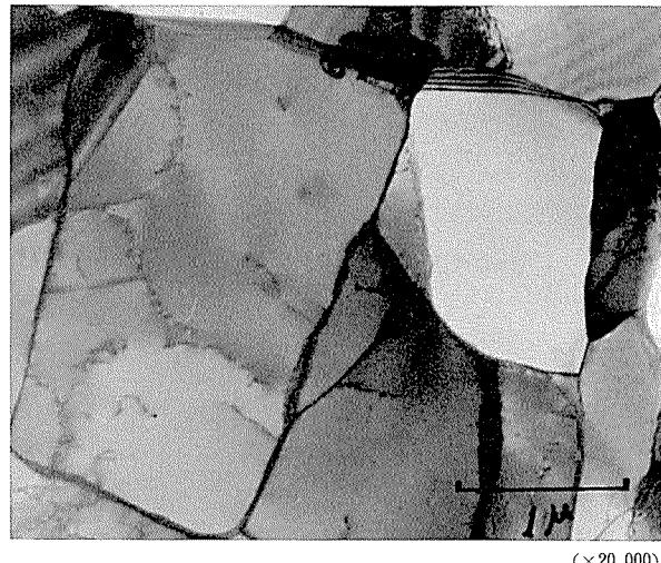
**Photo. 9** Transmission electron microstructure of commercial aluminum annealed at 250°C after 90% cold rolling.
