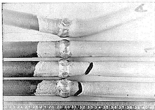
Photo. 5 TIG-welded tube joints between commercially pure aluminum and Zn-coated mild steel made with 1260 and 4043 filler rods after pressure and tensile tests.
