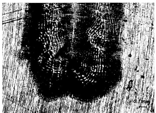
Photo. 8 Surface micrograph of the filiform corrosion generated on the pure aluminum sheet coated with vinyl paint.
