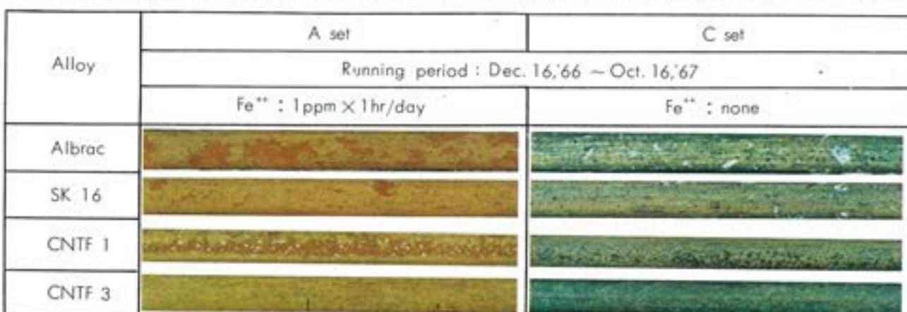
Photo. 4 Scale formed on the inner surface of tested tubes in A and C set.
