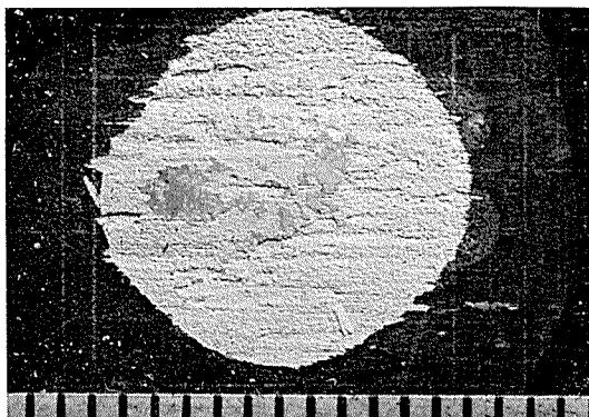
**Photo. 9** Corrosion occurred beneath the shell on the 1100 alloy specimen only pre-treated after 9 months dipped.
