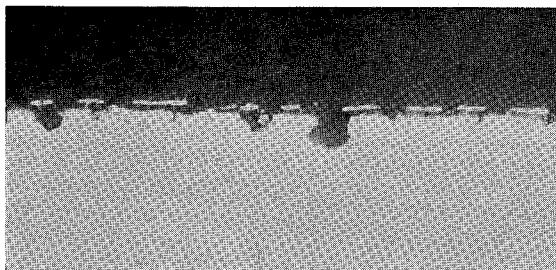
c) M.B.V. ( $1.9\mu$ )
