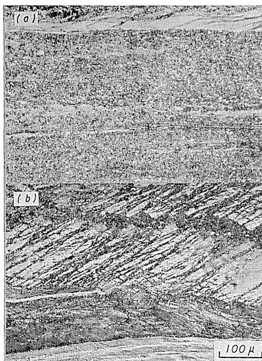
Fig. 9 Microstructures of 70-30 brass heavily cold rolled and then annealed at 250°C for 1 h.
