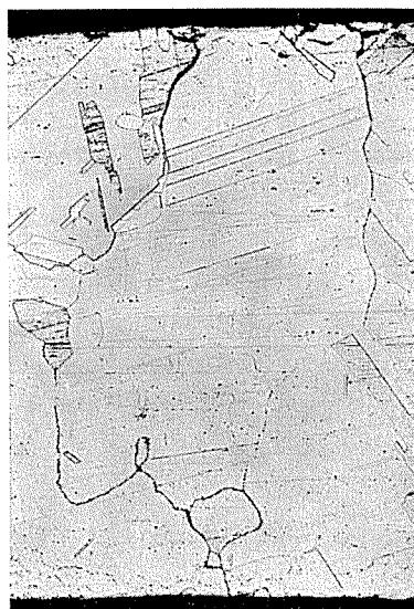
Fig. 2 Micro-structure of the phosphorus deoxidized copper tube failed with hydrogen embrittlement in a practical application. ( $\times 100 \times 2/3$ ) This tube contained  $0.004\%$  of phosphorus.
