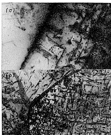
Fig. 11 Thin foil electron microstructures of (a) Al-8% Mg-0.2%Zr and (b) Al-8%Mg-0.3%Cu-0.2%Zr alloys water-quenched from 400°C and aged at 130°C for 30 days. ( $\times 4000$ )
