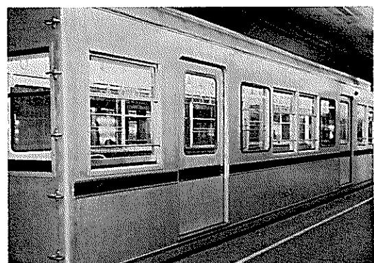
Fig. 26 Rolling-stock. (ZK60 and ZK61 alloys)
