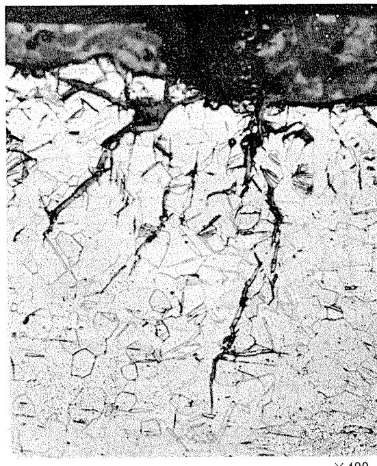
Fig. 9 Hydrogen absorption to form titanium hydride observed in titanium condenser tube used in sea water under cathodic protection by impressed current with potential -1.0~-1.4V v.s SCE.<sup>15)</sup>
