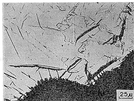
Fig. 4 Cross section of the corroded tube showing the hydride layer and needles at the bottom of the pit.
