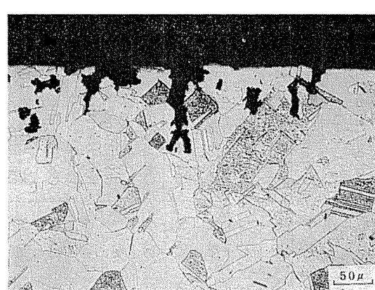
Fig.3 Formicary corrosion reproduced with 1.1.1-trichloroethane and water (specimen A12, after 7 days).
