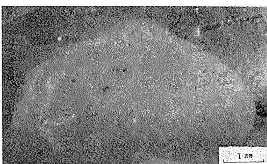
Fig. 1 Surface appearance of corroded copper tube in case No. 5.
