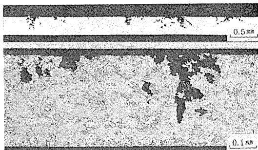
Fig. 2 Cross section of corroded copper tube in case No. 10.
