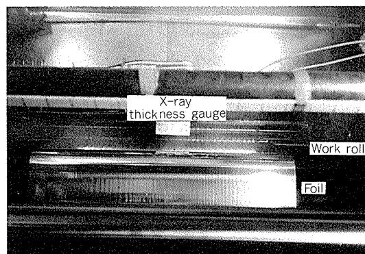
Fig. 2 Example of buckling wave in foil rolling.
