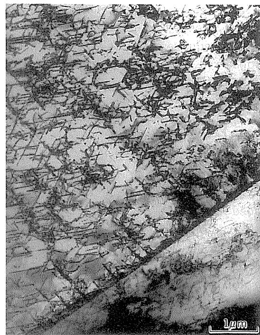
Fig. 8 TEM micrograph of the specimen having the grain size of 93  $\mu\text{m}$  deformed to 0.10 true strain.
