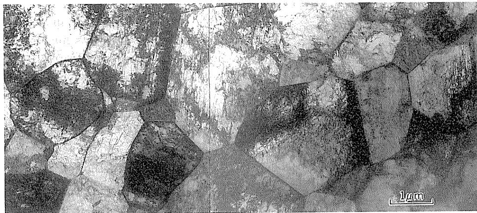
Fig. 3 TEM micrograph illustrating the uniform distribution of grains in the specimen having the finest ( $d = 1.6\mu\text{m}$ ) grain size deformed to 0.10 true strain.
